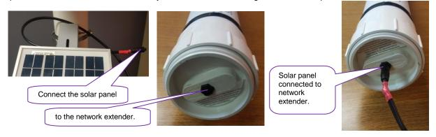
3. The network extender should wake up and activate on the base.
